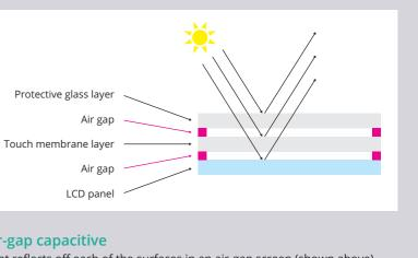
Light reflects off each of the surfaces in an air-gap screen (shown above) causing increased reflection. Sealing all three layers with optical adhesive eradicates the problem in true-bonded (shown below).
